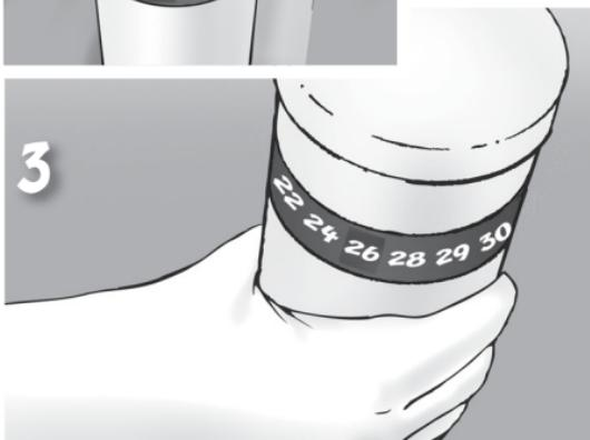
3. Remove the thermometer from the water and read the temperature (the number with the green background on the high-range thermometer). Record the number in degrees Celsius.
