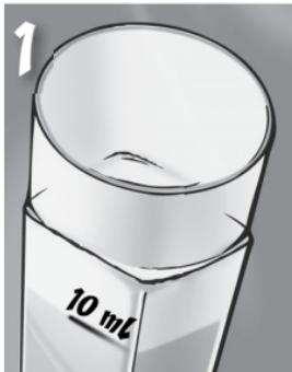
**1.** Fill the test tube (0106) to the 10 ml line with the water sample.
