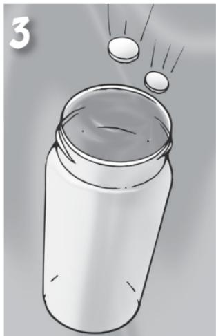
3. Drop two Dissolved Oxygen TestTabs® (3976) into the vial. Water will overflow when the tablets are added.
