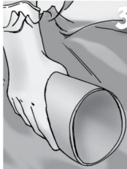
**3.** Hold the jar near the bottom and plunge it (opening downward) below the water surface.
