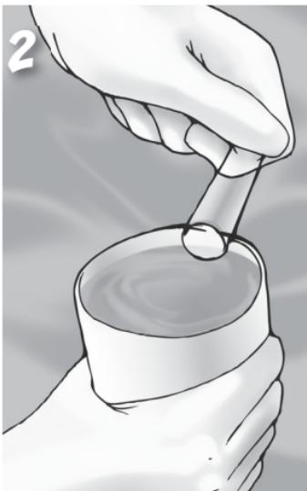
2. Submerge the small vial (0125) into the water sample. Carefully remove the vial from the water sample, keeping the vial full to the top.
