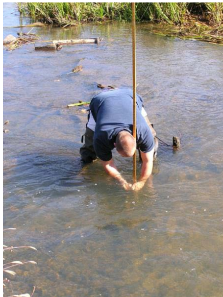
Figure 3. Capture of stratified water samples showing the use of a meter stick while opening sample bottle facing upstream and towards the water current.
