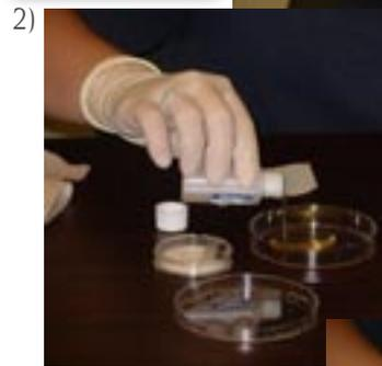
Volunteers used multiple test kits\* to determine the levels of *E. coli* in surface water samples.
